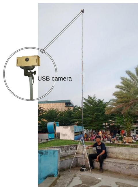
Figure 5. Field installation of the monitoring unit at Elephant Park
