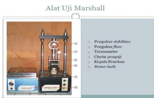
Gambar 1. Alat Uji Marshall
