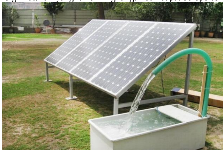
Gambar 7, Pompa air tenaga surya
